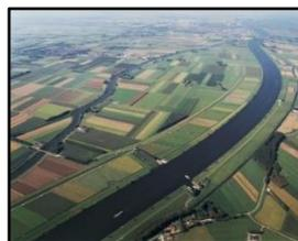
The Polder, on the south bank of the River Meuse, is one of over 30 'Room for the River' projects. Preventative measures were taken to enlarge the drainage capacity of the river during high water. So called 'river widening.'
